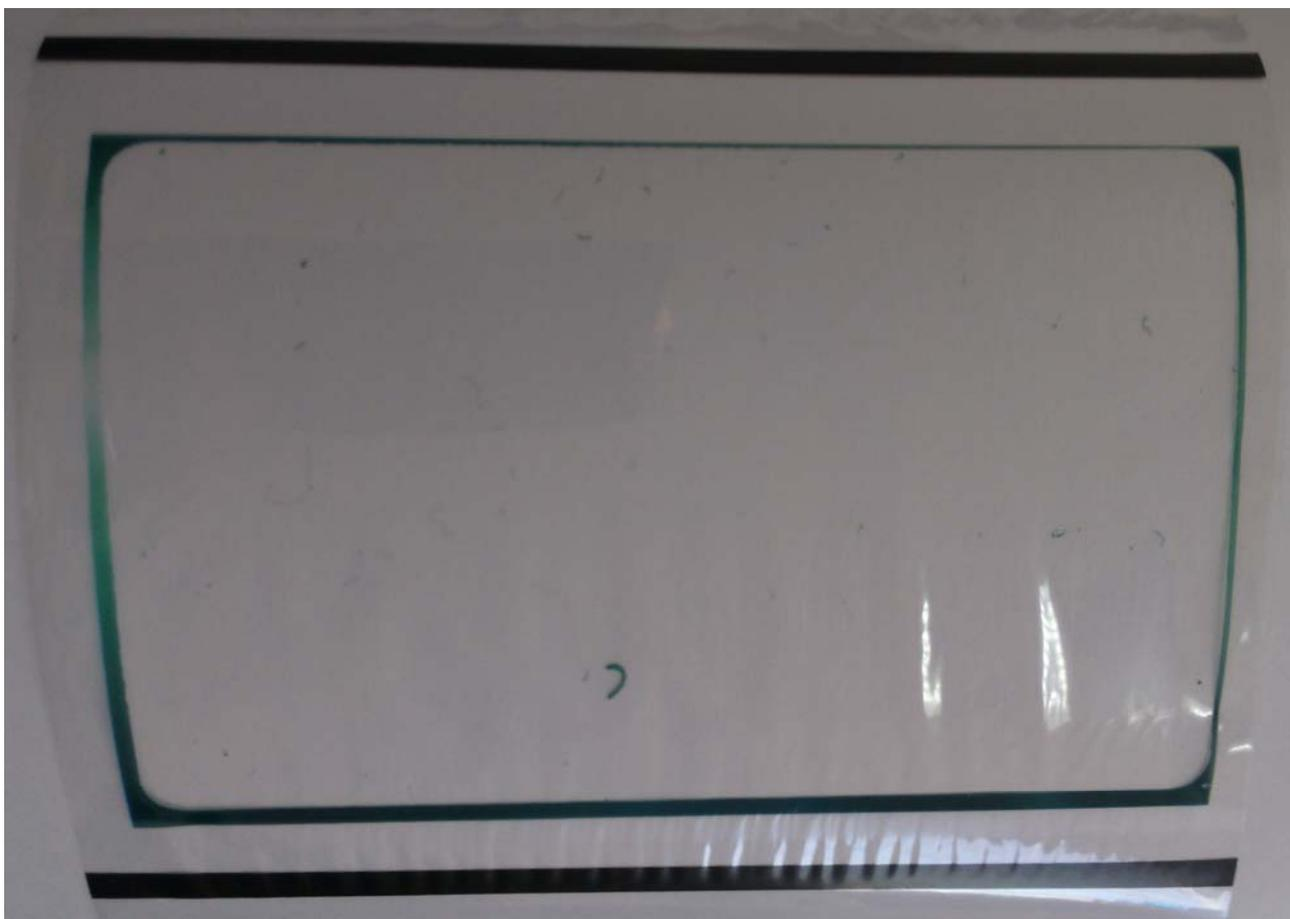
With printers like the Evolis Primacy, Datacard SD360, Zebra ZXP7 and others, they will leave a 1 to 2 mm unprinted area at the edges which is a limitation of the technology used in those printers. If we force the printer to print before the card is in position, the most likely outcome is a broken Ribbon or edges where we can peel the ribbon off of the card.
